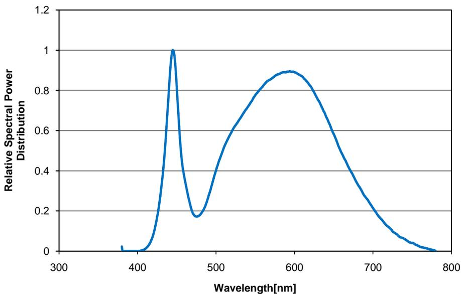
Cool White Relative Spectral Distribution vs. Wavelength Characteristic
