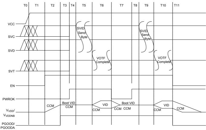
Figure 3. Simplified Sequence Timing Diagram
