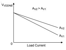
Figure 16. VDDNB Controller : Error Amplifier gain ( $A_V$ ) Influence on  $V_{VDDNB}$  Accuracy
