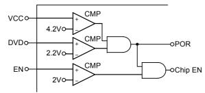
Figure 1. Power Ready (POR) Detection
