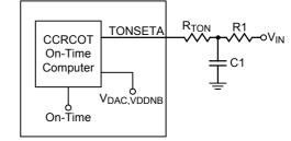
Figure 18. VDDNB Controller : On-Time Setting with  $\ensuremath{\mathsf{R}_{\mathsf{C}}}$  Filter
