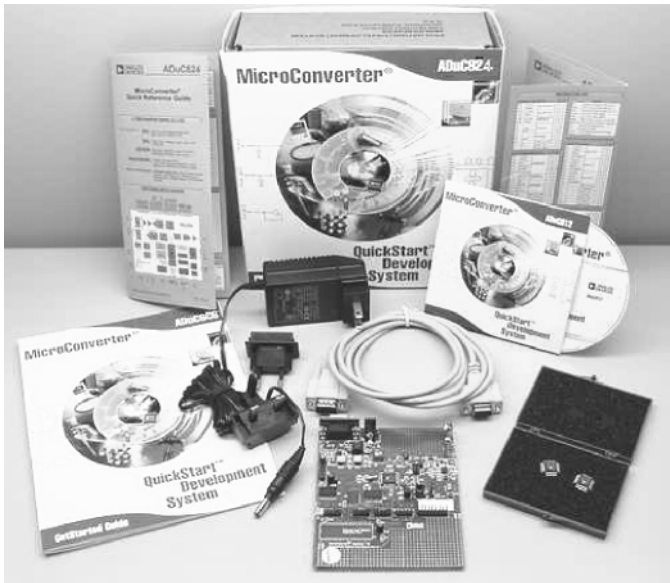
Figure 67. Components of the QuickStart Development System
