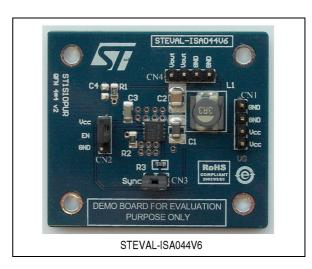
A thermal shutdown circuit is integrated and activates at 150 °C. Cycle-by-cycle current limitation provides protection against shorted outputs. The quiescent current is less than 6  $\mu$ A in the inhibit state.
