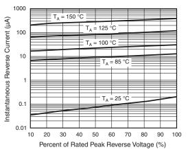
Figure 5. Typical Reverse Characteristics Per Diode
