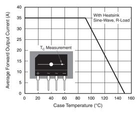
Figure 1. Derating Curve Output Rectified Current
