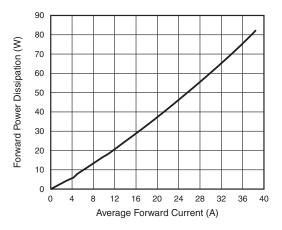
Figure 3. Forward Power Dissipation
