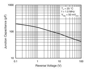
Figure 6. Typical Junction Capacitance Per Diode
