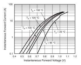
Figure 4. Typical Forward Characteristics Per Diode
