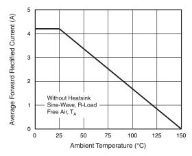
Figure 2. Forward Current Derating Curve
