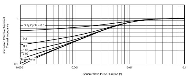
Normalized Thermal Transient Impedance, Junction-to-Case
