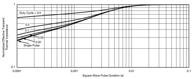
Normalized Thermal Transient Impedance, Junction-to-Case
