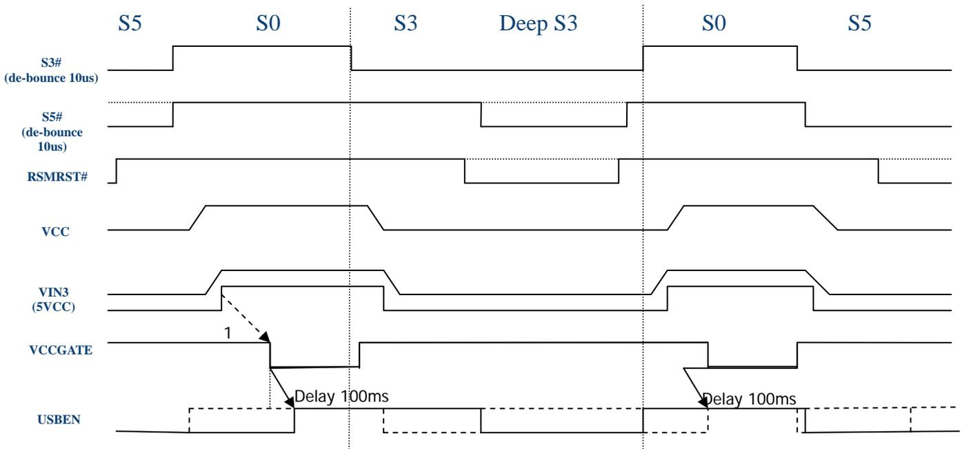
Figure 24 VCCGATE &amp; USBEN timing
