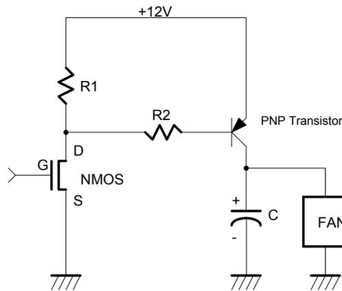
Figure 6 +12/5V PWM fan control application circuit
