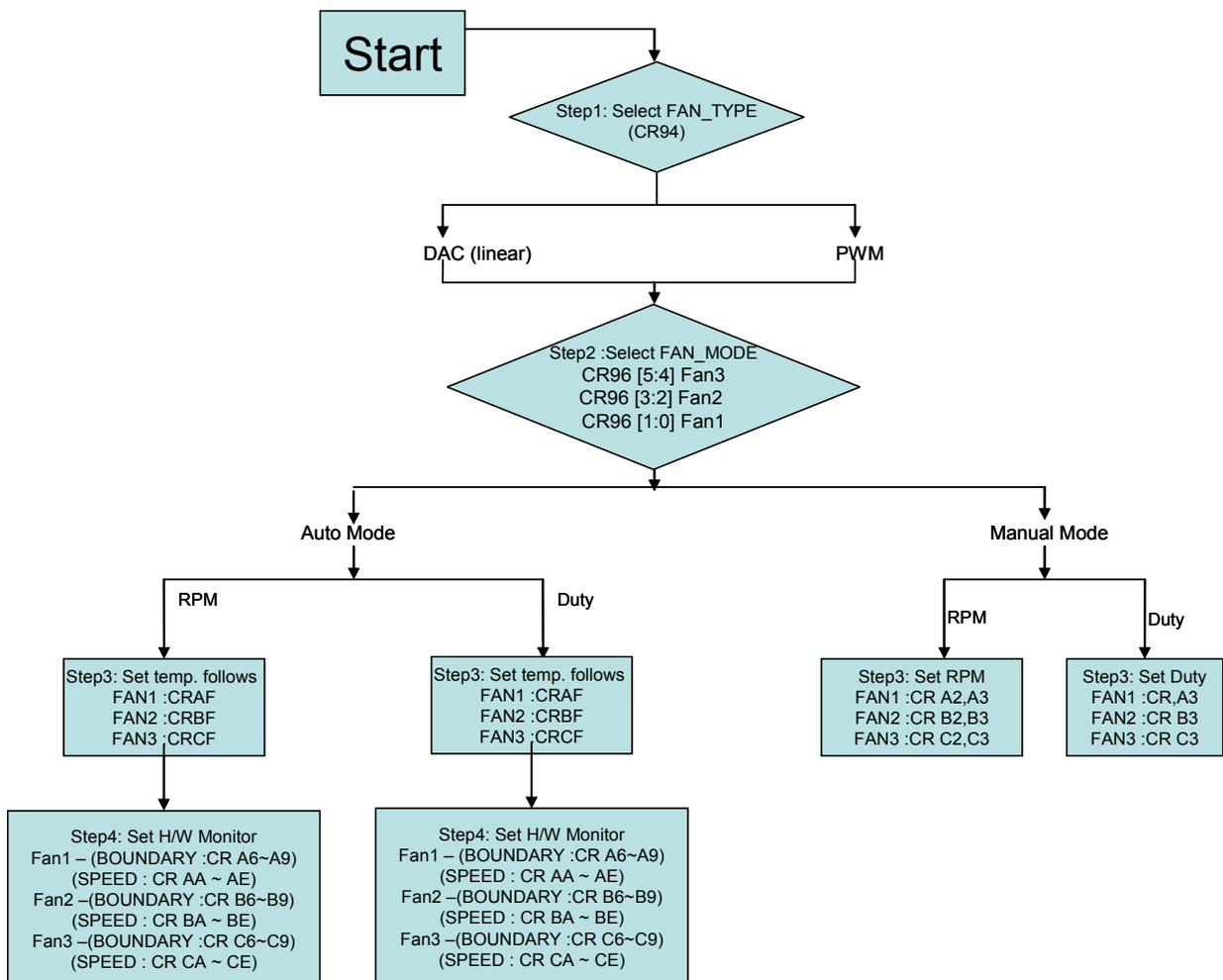
Figure 7 Fan type &amp; mode selection flow
