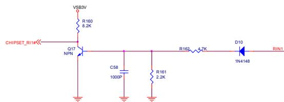
Wake up on ring for serial port circuit.
