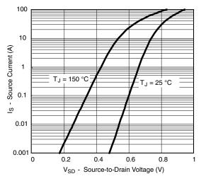
Forward Diode Voltage vs. Temperature
