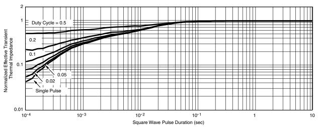
Normalized Thermal Transient Impedance, Junction-to-Case
