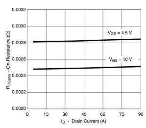
R<sub>DS(on)</sub> vs. Drain Current
