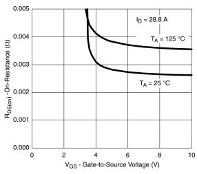
$R_{DS(on)}$  vs.  $V_{GS}$  vs. Temperature
