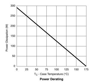
\*The power dissipation  $P_D$  is based on  $T_{J(max)} = 175$  °C, using junction-to-case thermal resistance, and is more useful in settling the upper dissipation limit for cases where additional heatsinking is used. It is used to determine the current rating, when this rating falls below the package limit.
