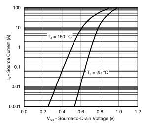
Source Drain Diode Forward Voltage
