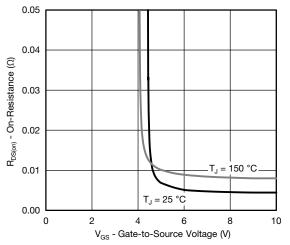
On-Resistance vs. Gate-to-Source Voltage
