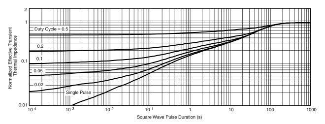
Normalized Thermal Transient Impedance, Junction-to-Ambient
