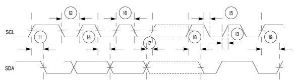
Figure 7. I<sup>2</sup>C Input/Output Timings
