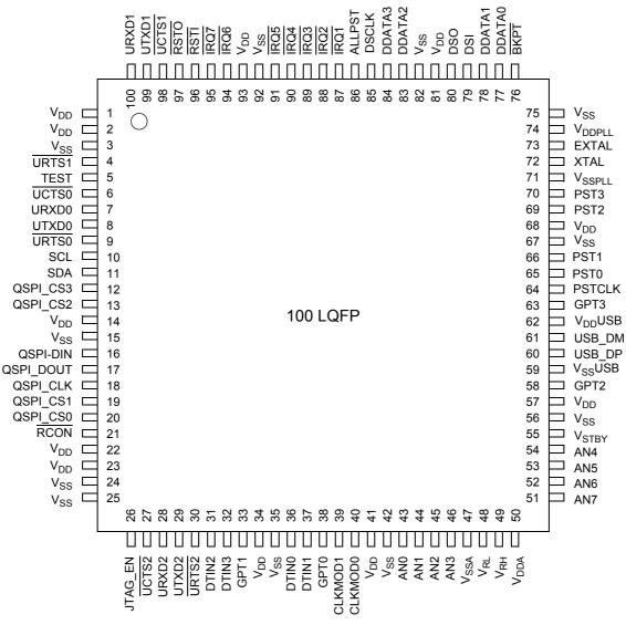
Figure 2. 100 LQFP Pin Assignments
