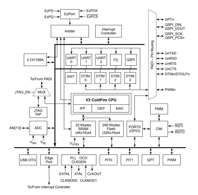
Figure 1. MCF52223 Block Diagram
