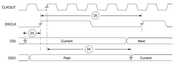
Figure 15. BDM Serial Port AC Timing
