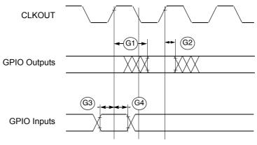
Figure 5. GPIO Timing
