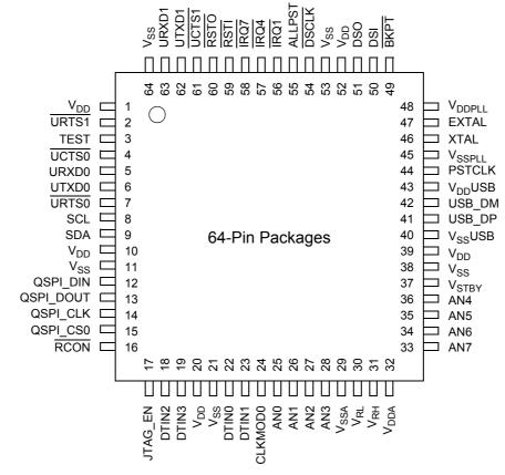
Figure 4 shows the pinout configuration for the 64 LQFP and 64 QFN.
