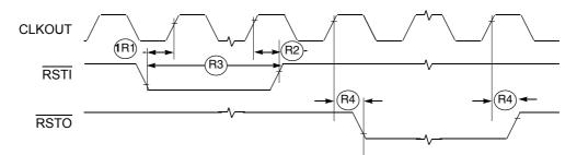
Figure 6. RSTI and Configuration Override Timing
