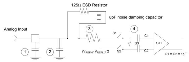
1. Parasitic capacitance due to package, pin-to-pin and pin-to-package base coupling; 1.8pF
