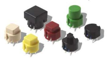
The D6 is a single-pole, momentary action, normally open keyswitch specially designed for digital electronic controls. Its small size enables keyboard design with minimum center spacing of 12.7 mm (0.500).
