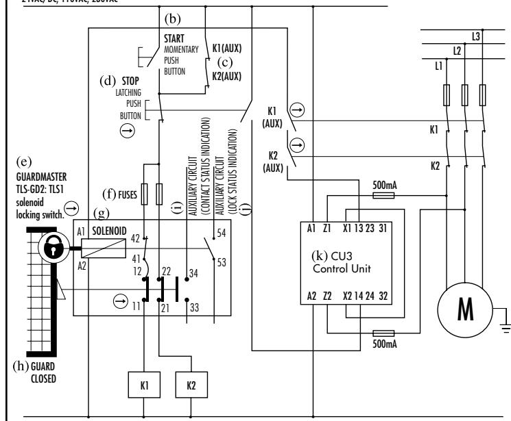
DO NOT EARTH (GROUND) 24V DC SUPPLY TO THE CU3. THIS MAY RESULT IN DAMAGE TO THE CU3.
