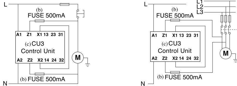
(d) The CU3 monitors the connections to the motor via the Z1-Z2 terminals. A break in the Z1-Z2 loop will be detected and the safety output contacts 13-14 & 23-24 will be prevented from closing when the motor is either running or stopped. To restore the CU3 function: isolate all power, repair the fault in the Z1-Z2 loop and reinstate power. Check for correct operation.
