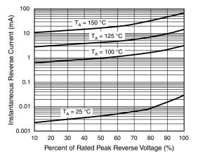
Fig. 4 - Typical Reverse Characteristics
