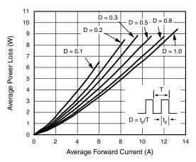
Fig. 2 - Forward Power Loss Characteristics
