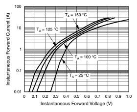
Fig. 3 - Typical Instantaneous Forward Characteristics
