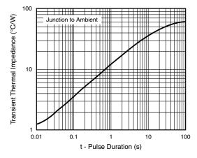
Fig. 6 - Typical Transient Thermal Impedance
