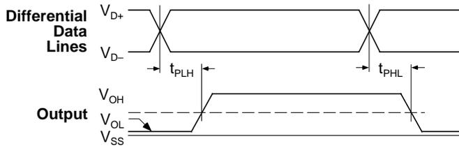
Figure 3. Receiver Propagation Delay D+/D- to RCV, V<sub>P</sub>, and V<sub>M</sub>
