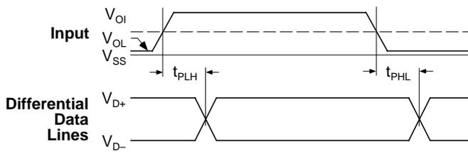
Figure 4. Driver Propagation Delay V<sub>P</sub> and V<sub>M</sub> to D+/D-
