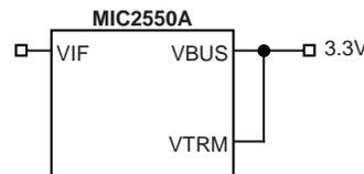
Figure 10. Powering Chip from Internal 3.3V Source
