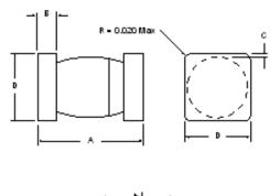
Note: Cathode side of device is indicated by a dark band marked on body.
