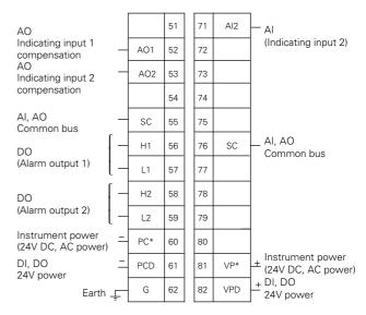
Note: \*Symbols for AC instrument power are VPO, PCO, approx. 24V DC (0.1A max.) output
