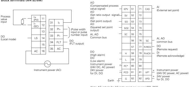
Note: \* Symbols for AC instrument power are VPO, PCO, approx. 24V DC (0.1A max.) output.
