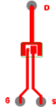
③ Mounted on minimum footprint full size board with metalized back and with small clip heatsink (still air)
