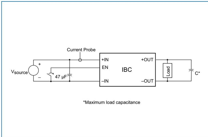
Figure 21 — Test circuit; inrush current overshoot
