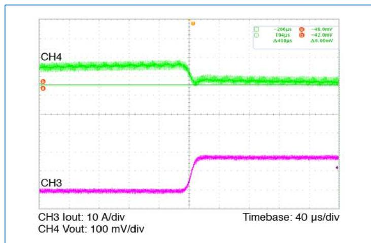
Figure 13 — Load transient response; nominal line
