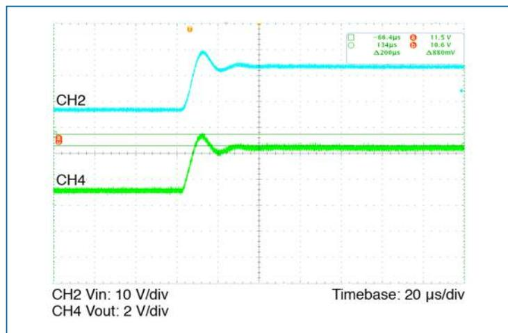
Figure 15 — Input transient response;
