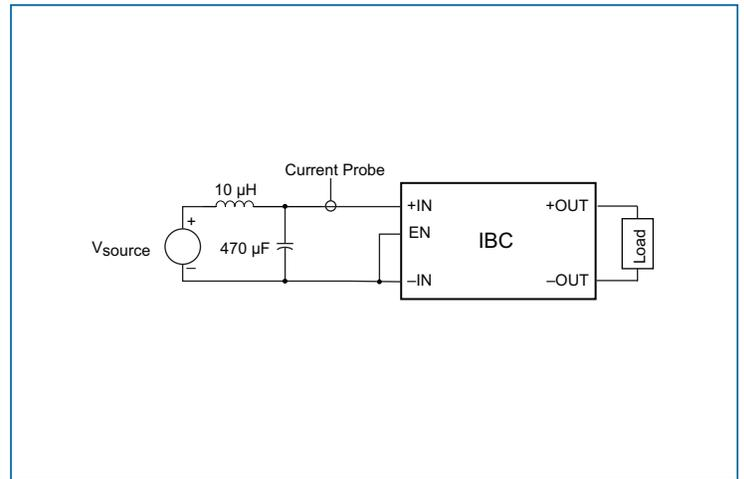
Figure 22 — Test circuit; input reflected ripple current
