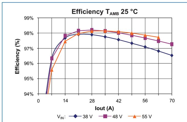
Figure 1 — Efficiency vs. output current, 25 °C ambient
