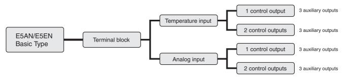
Note: Models with one control output or two control outputs can be used for heating/cooling control.
