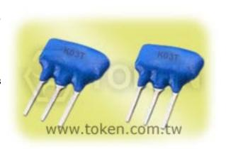
Token XT MT Ceramic Trap Filters (compatible to Murata TPT) series consist of 3 wafers with 3 trap frequencies. Recommended for Multi standard sets.
