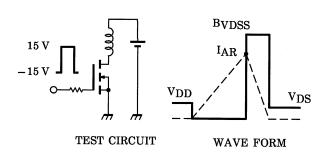
$$\begin{aligned} RG &= 25~\Omega \\ V_{DD} &= 25~V,~L = 213~\mu H \end{aligned} \qquad E_{AS} = \frac{1}{2} \cdot I \end{aligned}$$
