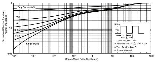
Normalized Thermal Transient Impedance, Junction-to-Ambient
