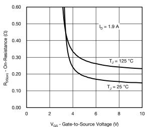
On-Resistance vs. Gate-to-Source Voltage
