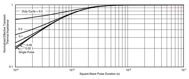
Normalized Thermal Transient Impedance, Junction-to-Case
