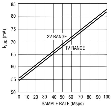
I_{VDD} vs Sample Rate, 5MHz Sine Wave Input, -1dB
