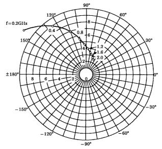
$\begin{array}{l} S_{12e} \\ V_{CE} = 8V \\ I_{C} = 5 \text{mA} \\ Ta = 25 ^{\circ}\text{C} \end{array}$
