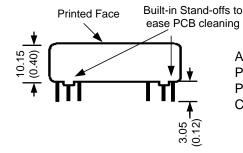
All dimensions are typical: millimeters (inches) Pin Diameter:  $0.50 \pm 0.05$  ( $0.02 \pm 0.002$ )
