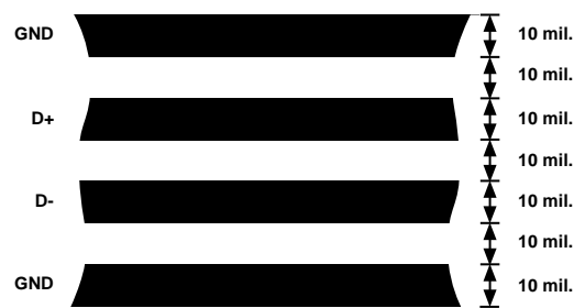
Figure 12. Arrangement of Signal Tracks
