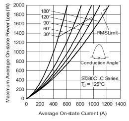
Fig. 5 - On-State Power Loss Characteristics
