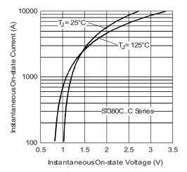
Fig. 9 - On-State Voltage Drop Characteristics
