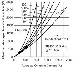
Fig. 6 - On-State Power Loss Characteristics
