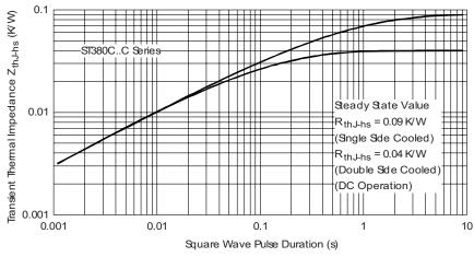
Fig. 10 - Thermal Impedance  $Z_{thJ\text{-}hs}$  Characteristics
