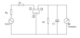
$\begin{array}{ll} R1=&280\,\Omega\pm5\%, R2=&330\Omega\pm5\%, Rg=&50\Omega & (1): Input\\ C2=&10 \mbox{ Pf} (Including stray capacitance & (2): Ground and capacitance of RF Voltmeter) & (3): Output\\ S.S.G: Output \mbox{ Voltmeter} & (3): Output \mbox{ Vol$
