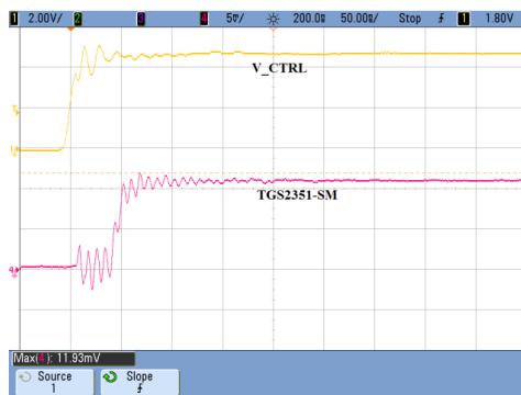
Switching Speed – On 50 ns Vc = 0/-40 V, Freq = 3 GHz, Pin = 30 dBm, +25 °C
