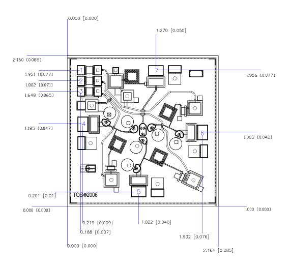
Units: millimeters (inches) Thickness: 0.100 (0.004)
