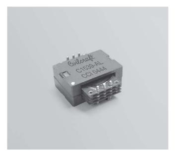
The C1539-AL was developed specifically for the National Semiconductor LM5032 dual interleaved current mode PWM controller. This planar transformer can be used in a dual forward converter or in both interleaved power stages of a high-current converter in applications up to 100 Watts.
