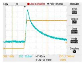
Figure 1: Startup Pop-Noise without PA4220 (32 Ω load)
