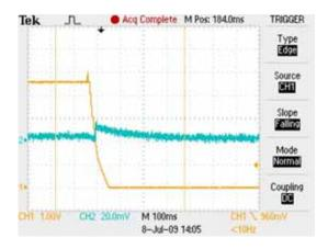
Figure 4: Shutdown Noise with PA4220 (32  $\Omega$  load)
