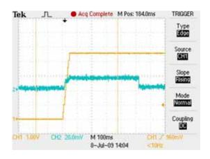
Figure 2: Startup Pop-Noise Reduction with PA4220 (32  $\Omega$  load)
