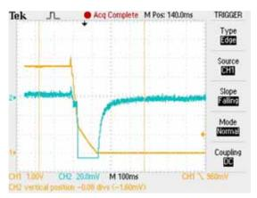
Figure 3: Shutdown Noise without PA4220 (32 Q load)
