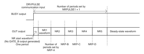
For example, when NRPULSE1 is set to 15, NRP-A to 3, NRP-B to 6, NRP-C to 9, and NRP-D to 12, one period of the NR start waveform (no GATE\_B output) is output, followed by three periods of the NR1 waveform, three periods of the NR2 waveform, three periods of the NR3 waveform, three periods of the NR5 waveform, and then STP x DRVPULSE periods of the steady-state waveform.
