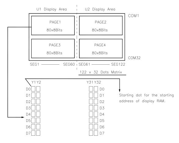
Each segment driver has 4 pages RAM, and each page has 80x8 bits RAM.  $D0\sim D7$  are 8 bits transmitted data, where D0 is LSB and D7 is MSB.
