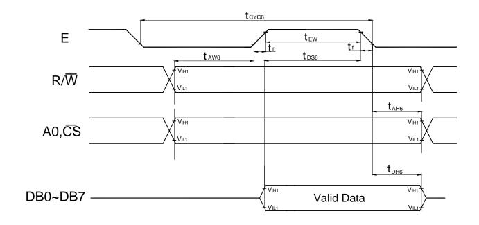
Fig. b Interface timing (data Write)
