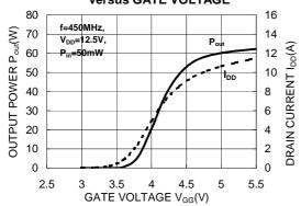
RoHS Compliance, 400-450MHz 45W 12.5V, 3 Stage Amp. For MOBILE RADIO
