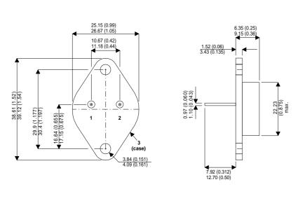
Bipolar PNP Device in a Hermetically sealed TO3 Metal Package.
