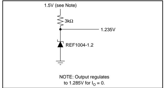
FIGURE 3. 1.2V Reference from 1.5V Battery.
