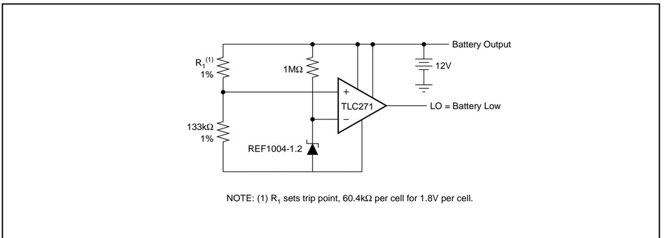
FIGURE 5. Lead-Acid Low-Battery-Voltage Detector.
