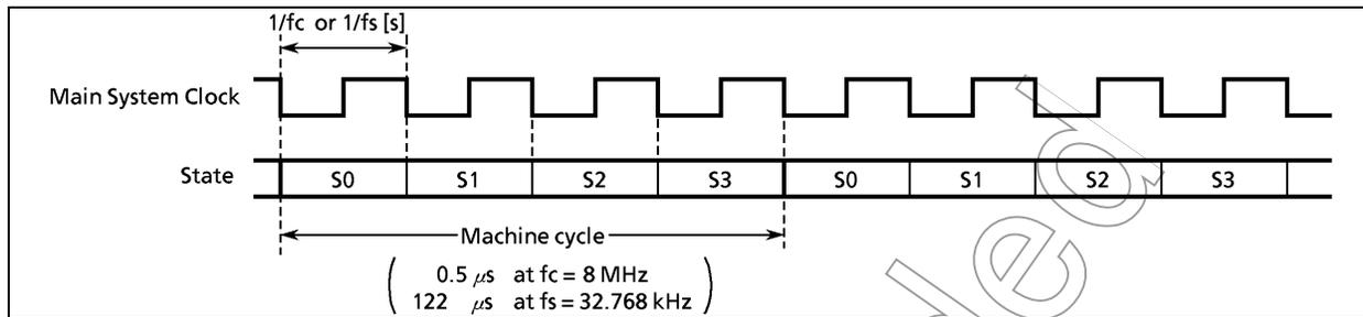
Figure 1-13. Machine Cycle
