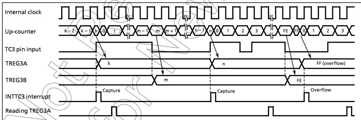
Figure 2-28. Timing Chart for Capture Mode (INT3ES = 0)
