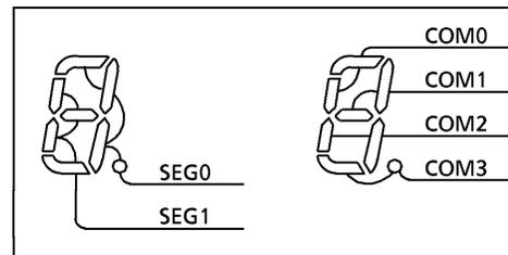
Figure 2-48. Example of COM, SEG Pin Connection (1/4 Duty)
