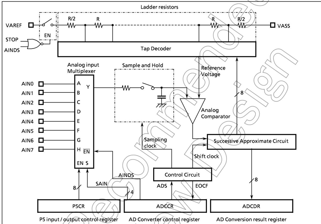
Figure 2-55. AD Converter
