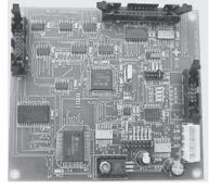
The PDS-500/-1 is a plasma graphic display controller which can drive a variety of popular plasma displays having a common 14 pin video interface. The controller can clock displays with 128 x 32, 128 x 64, 192 x 64, 256 x 64, and 320 x 64 pixel formats. When integrated with a display and optional DC/DC converter, the ASCII input graphics controller is the final ingredient needed to form a highly reliable, rugged, slim profile DC plasma display sub-system.
