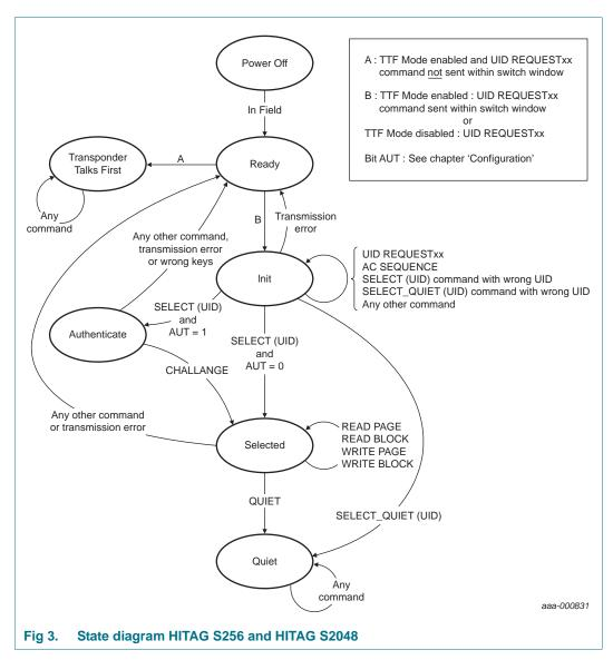
**Remark:** Switching off the powering magnetic field or moving the HITAG S Transponder out of the RWD antenna field enters the HITAG S Transponder into the Power off state independently of its actual state.
