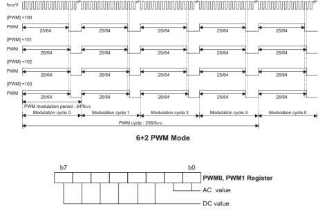
6+2 Pulse Width Modulation Mode Registers
