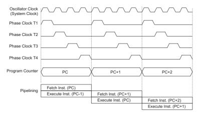
System Clocking and Pipelining
