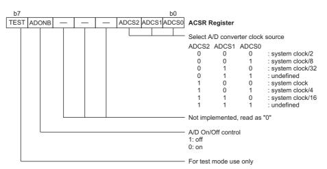
A/D Converter Clock Source Register
