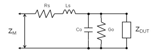
$Z_M$  is defined as total impedance measured to DUT by the special test fixture which has some parasitic impedance.  $Z_M = (Rs + j\omega Ls) + (\frac{1}{Go + j\omega Co} \parallel Z_{DUT})$
