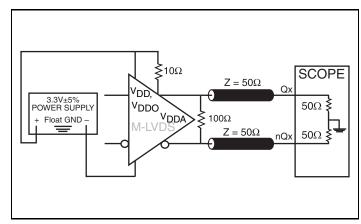
3.3V M-LVDS Output Load AC Test Circuit
