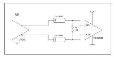
Figure 4D. HiPerClockS CLK/nCLK Input Driven by a 3.3V LVDS Driver
