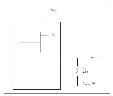
Figure 9. LVPECL Driver Circuit and Termination
