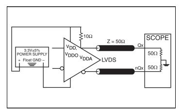
3.3V LVDS Output Load AC Test Circuit
