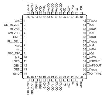
ICS8743008I 56-Lead VFQFN 8mm x 8mm x 0.925mm package body K Package Top View
