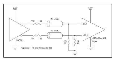
Figure 4E. HiPerClockS CLK/nCLK Input Driven by a 3.3V HCSL Driver
