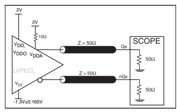
3.3V LVPECL Output Load AC Test Circuit
