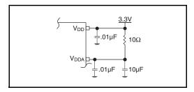
Figure 2. Power Supply Filtering
