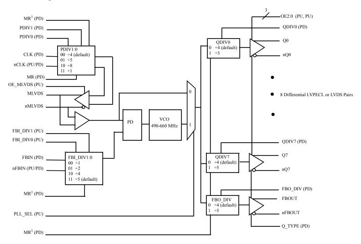
One master reset pin is used to reset all the internal dividers, but the MR lines are not drawn as all tied together to reduce control line clutter, making the block diagram easier to read
