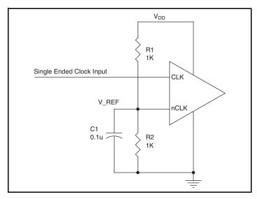
Figure 3. Single-Ended Signal Driving Differential Input
