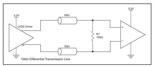
Figure 6. Typical LVDS Driver Termination
