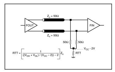
Figure 8A. 3.3V LVPECL Output Termination
