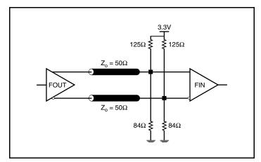
Figure 8B. 3.3V LVPECL Output Termination
