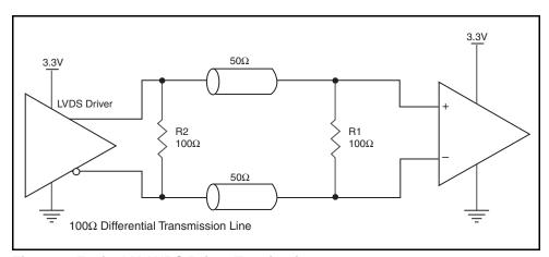
Figure 7. Typical M-LVDS Driver Termination
