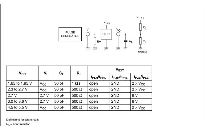
$C_L$  = Load capacitance including jig and probe capacitance.
