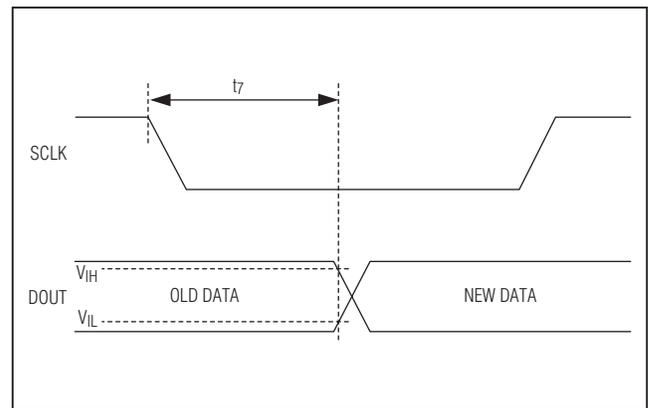
Figure 3. Hold Time After SCLK Falling Edge
