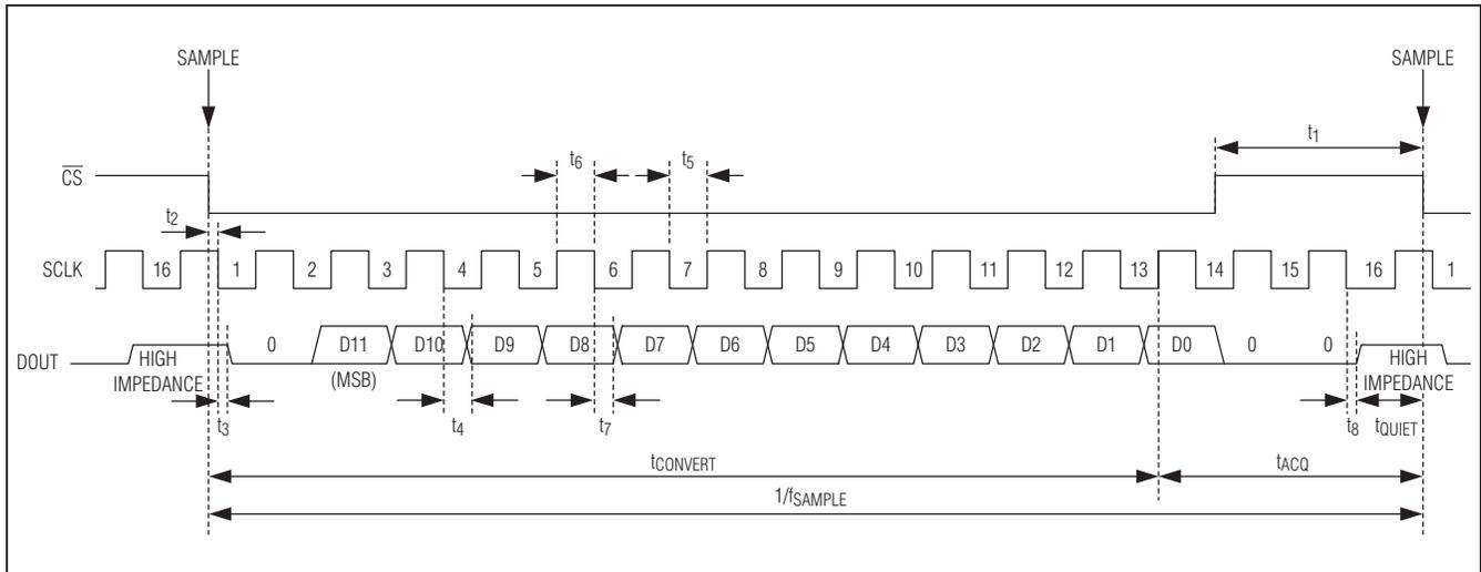
Figure 1. Interface Signals for Maximum Throughput, 12-Bit Devices
