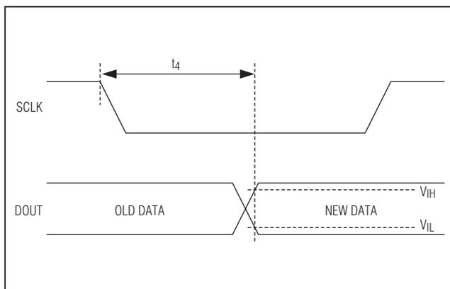
Figure 2. Setup Time After SCLK Falling Edge
