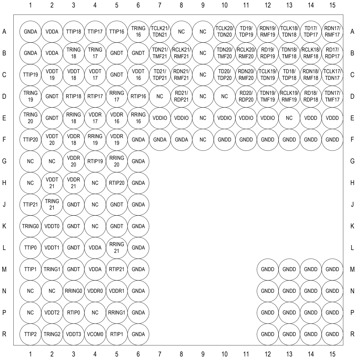
Figure-3 640-Pin TEPBGA (Top View) - Top Left
