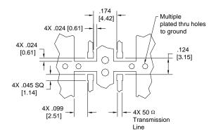
Dimensions are in Inches [Millimeters] 1P503\* Mounting Footprint
