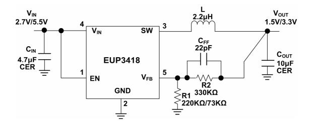
Figure 1. Adjustable Output
