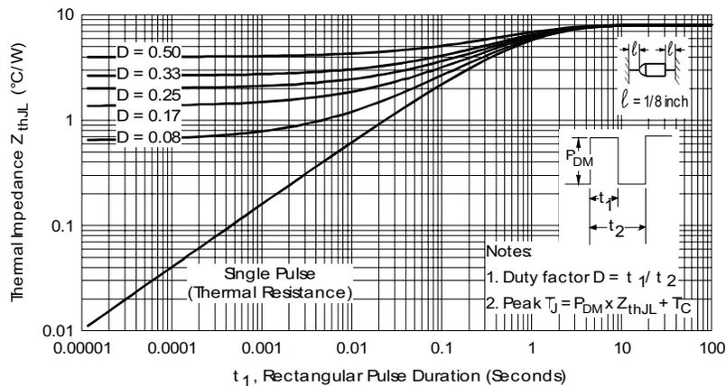
Fig. 4 - Maximum Thermal Impedance  $Z_{thJL}$  Characteristics
